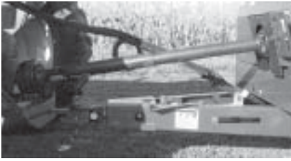
Telescoping PTO Drive (3 zerks)
