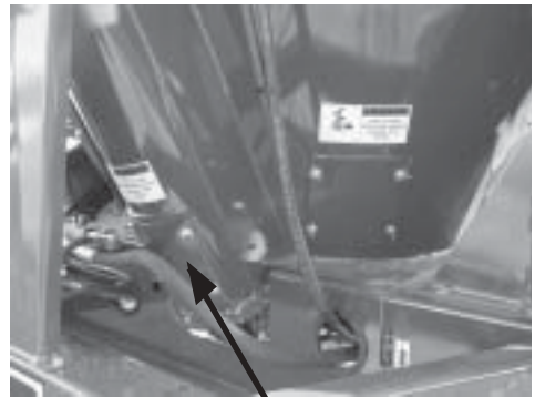
Lower Unloading Auger Cleanout
