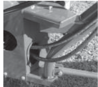
SIA Upper Pivot Bearing (1 zerk) SIA Lower Pivot Bearing (1 zerk)
