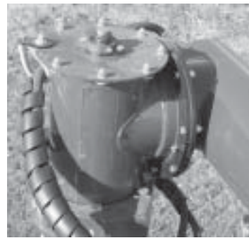
Unloading Auger(1 zerk on the top of vertical section auger and 4 zerks on vertical auger pivot.)
