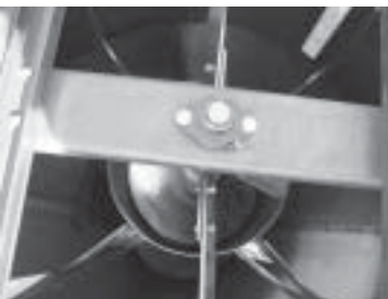
Top of Mixing Auger (1 zerk - under top of tank cover)
