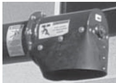
Unloading Auger-(1 zerk at the end of the auger discharge spout)
