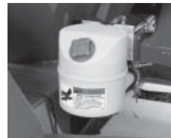
Oil level should be between Max/Min level marks
