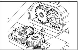
The name-plate on the cover gives the number of teeth of the gear pair originally installed by the Manufacturer, furthermore, as on page 4 of this handbook, there are the speeds pertaining to the pairs of gears monuted on purchase, plus of the spare pairs.
